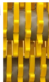
This is the intermediate fragment kit. Combs are fitted to the system and it is denoted by grey rings.
